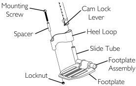
FIGURE 4.7 Replacing Heel Loop
